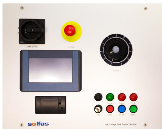
Picture GHV control unit operation panel
